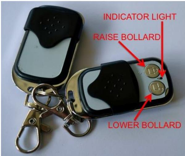
Point your remote control in the direction of your bollard and press the left “lock” button to raise your bollard into the upright position
